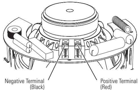
Press down on the terminal tab to open the hole; insert the bare end of the wire into the hole; and release the tab to secure the wire. NOTE: C383XC and C363XC models have post-type terminals. Press down on the post to open the hole; insert the bare end of the wire into the hole and release the post to secure the wire.
